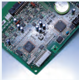
Optimum control software 1 High-speed switching control: DSP 2 System total control: CPU
